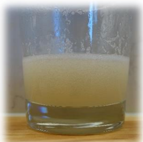
Sunflower oil and water mix, before and after beet pectin was added, with mix heated to 50-55°C.
